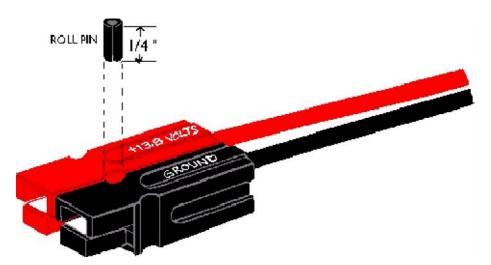
Housings should be mated according to the diagram above, viewing from the contact side (opposite the wire side), tongue down, hood up, *red* on the left, *black* on the right. Use a 3/32-inch-diameter roll pin, 1/4 inch long, to keep the housings from sliding apart.
